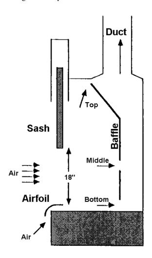
**Sash**- The sash is the glass "window" that travels in the plane of the hood face that opens or closes the hood and protects the user during use.
