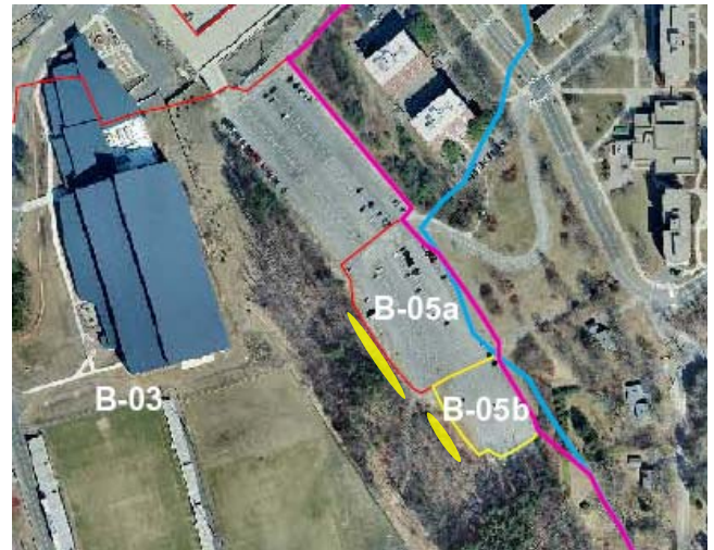
Figure 1. Drainage areas to two proposed bioretention cells.
