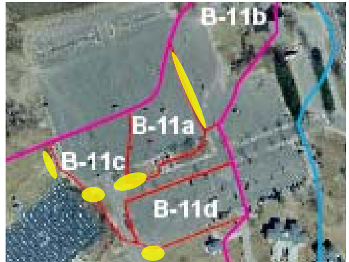
Figure 1. Location of proposed bioretention cells. Two portions of lot drain out of the Eagleville Brook watershed (outside of pink line).
