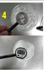
If the dial thermometer is not at  $32^{\circ}F(0^{\circ}C)$ , with the thermometer still in the ice water, twist the nut on the back of the dial until the needle on the dial reaches  $32^{\circ}F(0^{\circ}C)$
