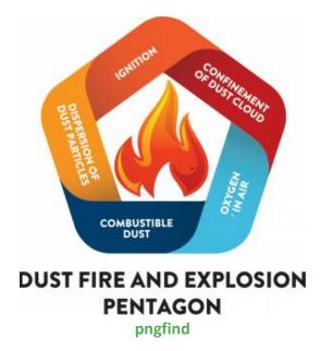
When all five conditions are met, an initial dust explosion in equipment can cause accumulated dust to become airborne. If the airborne dust is ignited, it may cause one or more secondary explosions that can be more destructive than the primary explosion.
