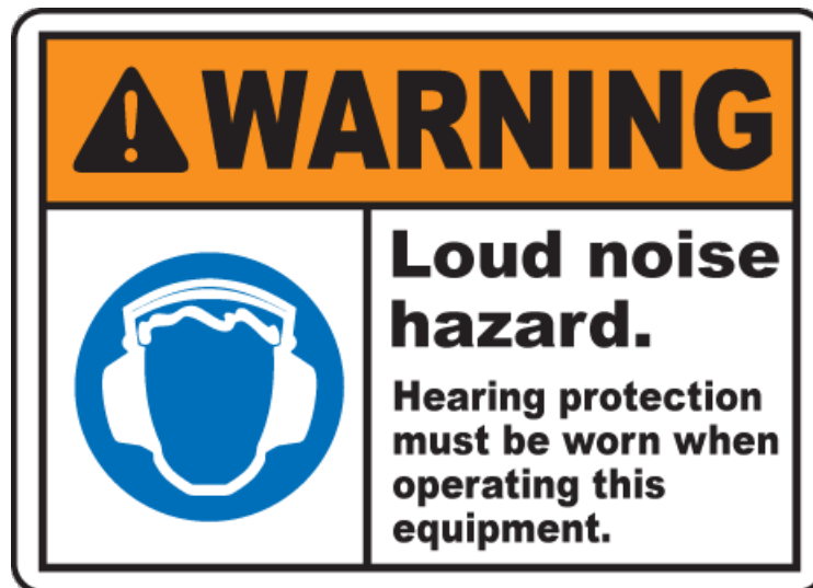
Example of Loud Equipment Sign
